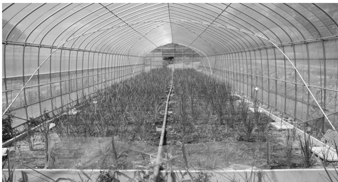
Fig. 3 Watertight experimental bed installed with line source sprinkler system, which creates and maintained various intensities of soil moisture stresses.
