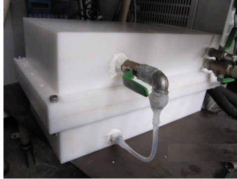
Figure 2 All-in-one type adsorption heat pump prototypes
