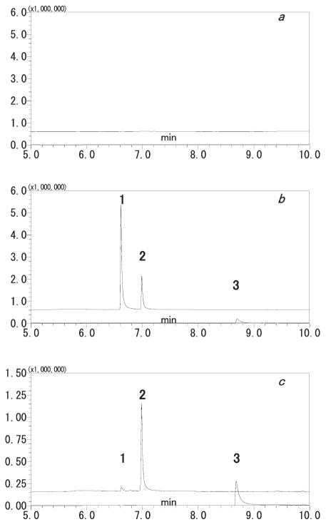
Fig. 2 Selected ion monitoring (SIM) chromatograms for nicotine (1), IS (2), and cotinine (3) extracted from human urine. In Fig. 2*b*, nicotine, IS, and cotinine were spiked into blank human urine samples at concentrations of 100, 500, and 1000 ng/mL, respectively.
