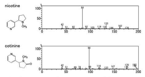
Fig. 1 Chemical structures and electron ionization mass spectra of nicotine and cotinine.
