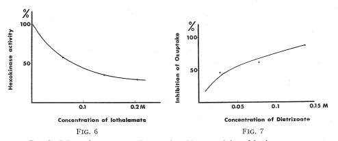
FIG. 6. Effect of contrast medium on hexokinase activity of brain. Reaction medium contained 0.15 M MgCl<sub>2</sub> (final  $5 \times 10^{-3}$  M), 0.1 ml of 1.0 M ATP and 0.4 ml of homogenate. Inhibition rate means the ratio of dosis of glucose consumption in the presence of Diatrizoate to that in the absence of it.
