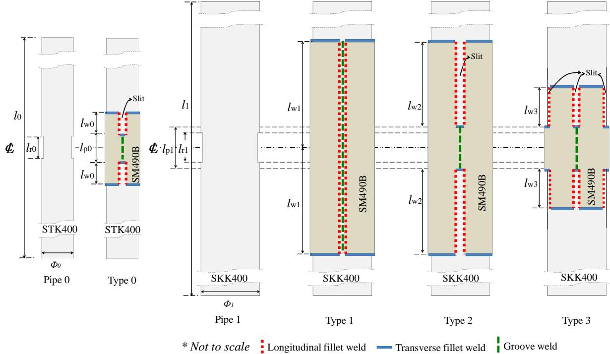
**Figure 4: Examined pipes and repaired types**
