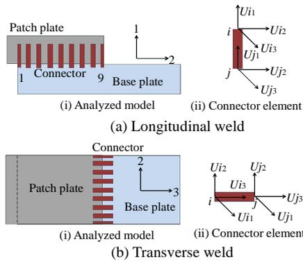
Figure 1: Weld model
