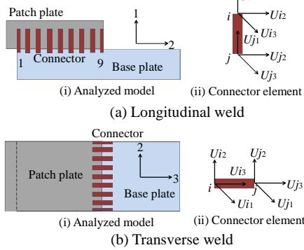
**Figure 1: Weld model**
