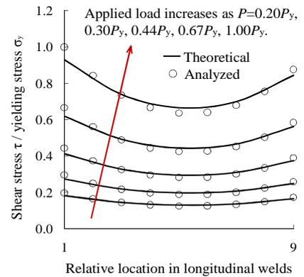
Figure 3: Shear stress distributions
