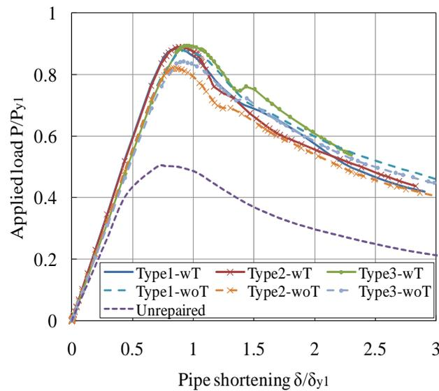
**Figure 8: Global responses between different repaired types**
