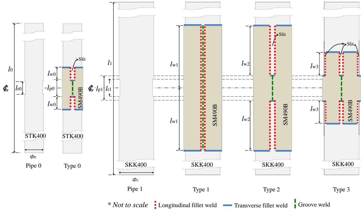
**Figure 4: Examined pipes and repaired types**
