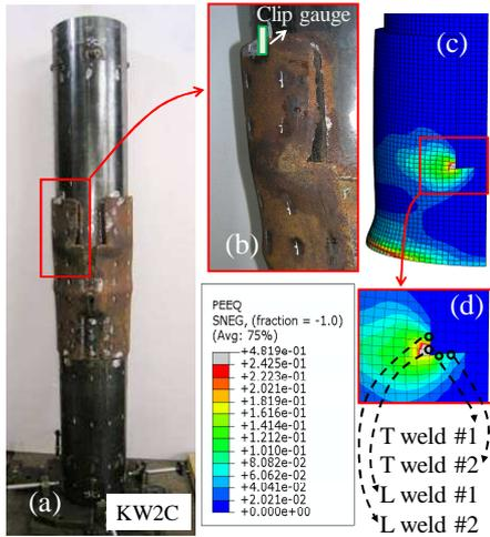
**Figure 6: Comparison of failure modes**
