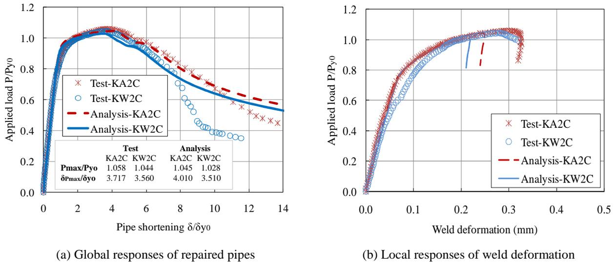
**Figure 5: Comparisons of validation tests on repaired pipe Type 0**
