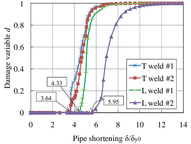
**Figure 7: Damage progress of welds in KW2C**
