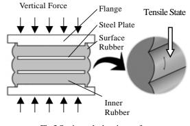
Fig.3 Strain on the bearing surface
