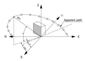
Fig.14 Angle diagram for finding solar radiation on vertical surfaces
