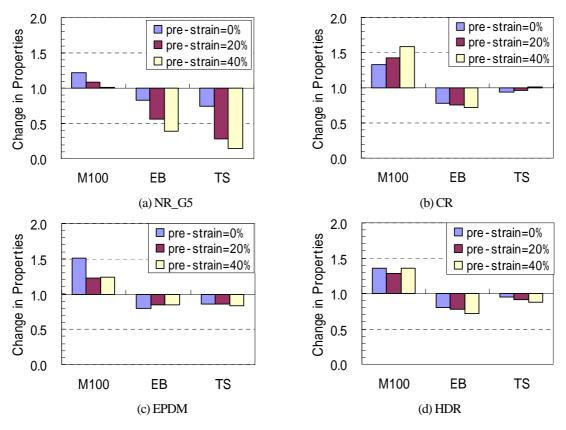
Fig.8 Influence of pre-strain on ultraviolet deterioration (720 hours)
