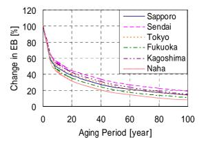
Fig.17 EB degradation of CR coating in the shadow
