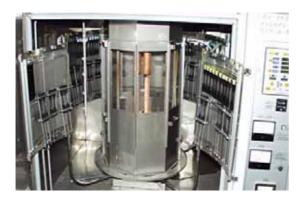
Fig.5 Dew cycle sunshine weather meter
