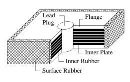
Fig.1 Bridge rubber bearing
