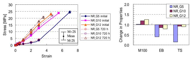
Fig.11 Aging characteristics of NR subjected ultraviole irradiation (pre-strain=40%)
