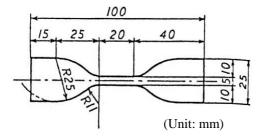
Fig.2 JIS No.3 dumbbell specimen
