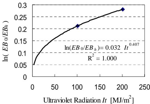
Fig.13 Relationship between EB change in CR and ultraviolet intensity
