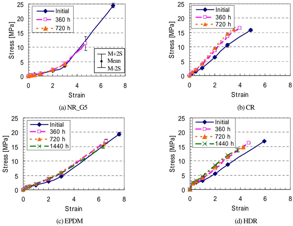
Fig.6 Effect of ultraviolet irradiation on rubber mechanical properties (pre-strain=40%)
