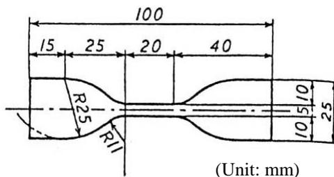
Fig.2 JIS No.3 dumbbell specimen
