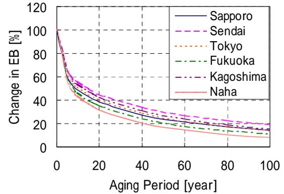
Fig. 17 EB degradation of CR coating in the shadow
