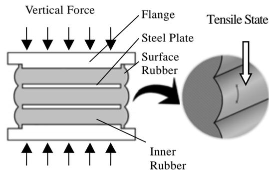
Fig.3 Strain on the bearing surface
