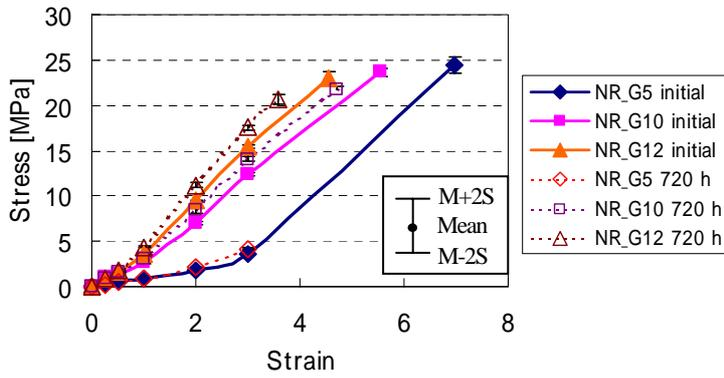
Fig.11 Aging characteristics of NR subjected ultraviolet irradiation (pre-strain=40%)
