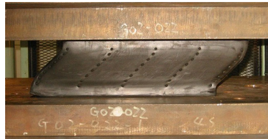
Fig. 4 Cyclic test of HDR bearing for 175% shear strain
