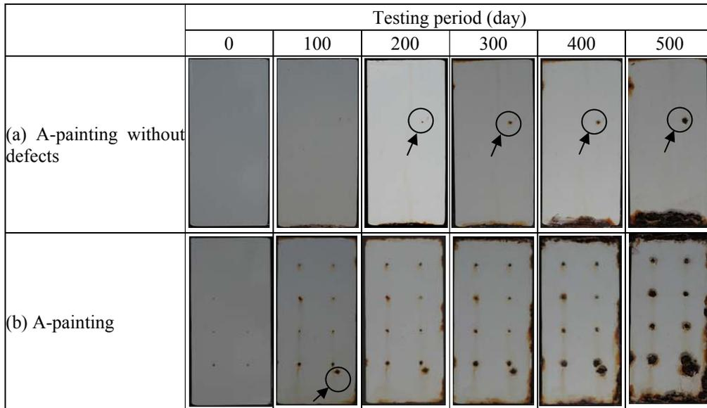
**Figure 3. Appearance change in A-painted specimens**
