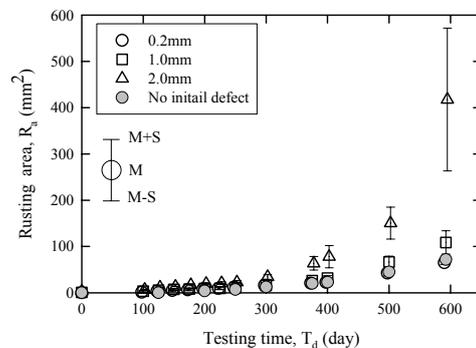
**Figure 5. Rust areas of A-painted specimens**
