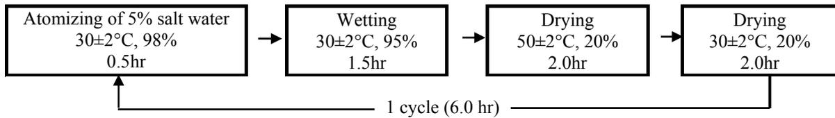
**Figure 2. S6-cycle test condition**
