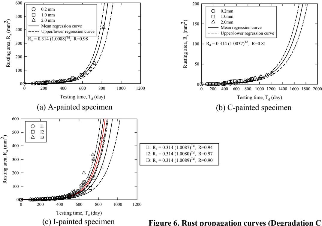
Figure 6. Rust propagation curves (Degradation Curves)
