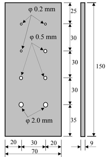
Figure 1. Test specimen (mm)
