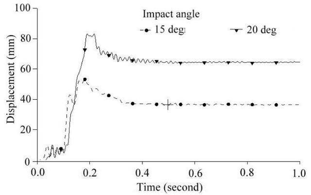
Fig. 7 Displacement – time history of railing post (curved railing with 150 m of radius)
