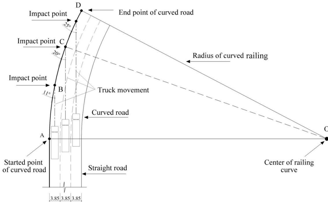
Fig. 5 Impact angle of truck and railing on the curved roads and bridges
