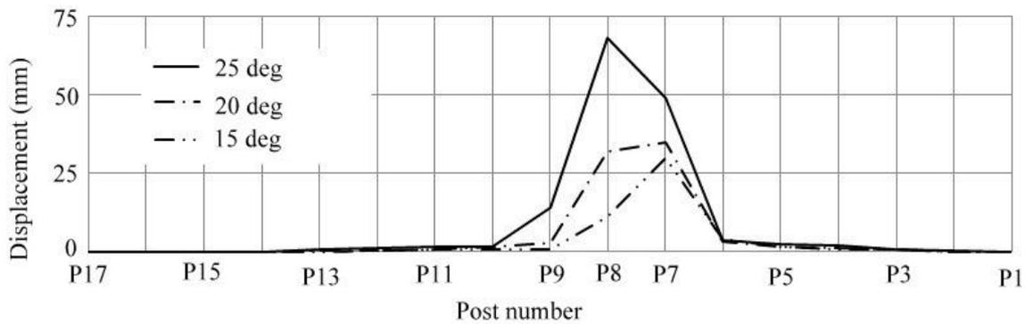
Fig. 8 Lateral deformation of railing (curved railing with 100 m of radius)
