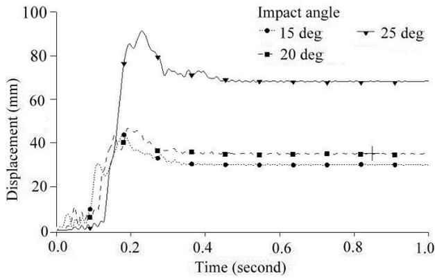
Fig. 6 Displacement – time history of railing post (curved railing with 100 m of radius)
