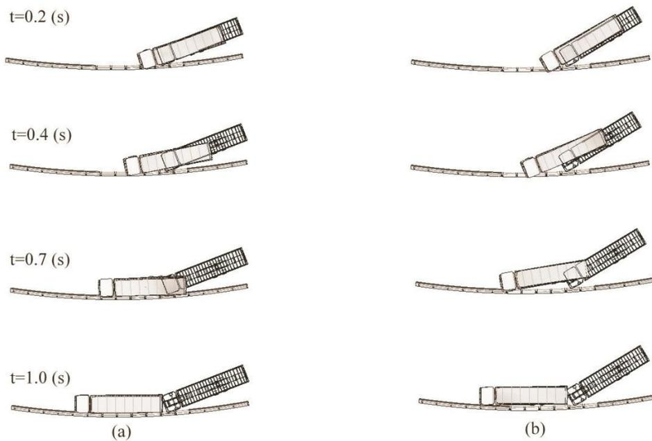
Fig. 9 Truck movement for curved railing with 100 m of radius (a) 15 degree of impact angle, and (b) 25 degree of impact angle
