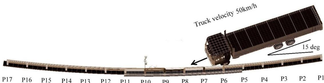
**Fig.2** The 3D model of impact collision between truck and railing
