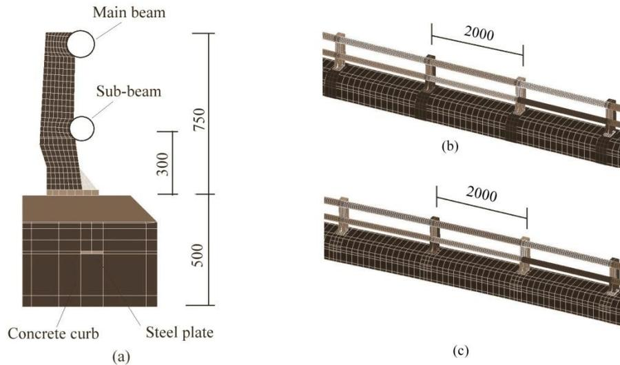
**Fig.1** FE models of railing (Unit: mm), (a) Cross section, (b) Straight railing, and (c) Curved railing
