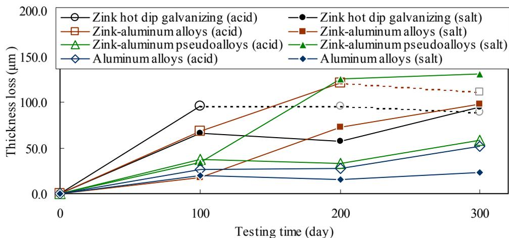
Figure 5: Thickness Loss of Metallic Coating Systems
