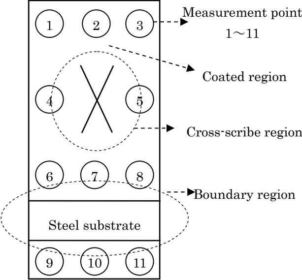
Figure 3: Classification of Regions in a Test Specimen and Thickness Measurement Points
