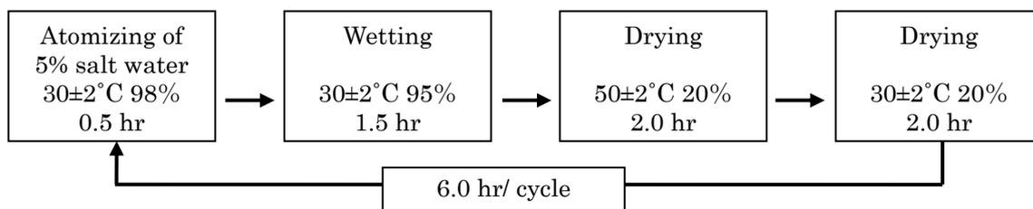
(a) Salt water spray combined cyclic test
