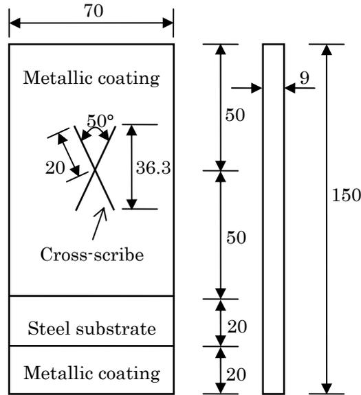
Figure 1: Geometry of the Test Specimens
