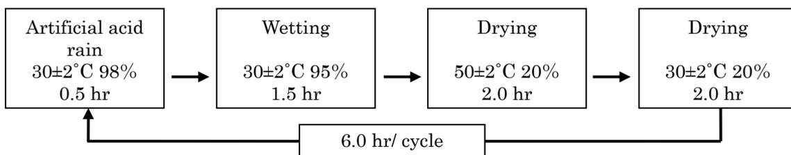
(b) Acid rain spray combined cyclic test
