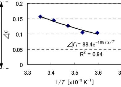
Figure 5: Temperature dependency of  $\Delta f_i$
