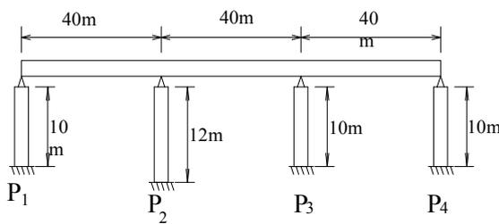
Figure 7: Base-isolated multi-span continuous bridge example
