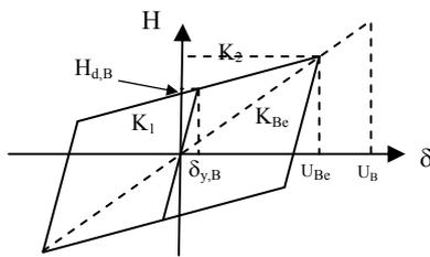
Figure 9: Bilinear force-displacement relationship of HDR bearing stiffness
