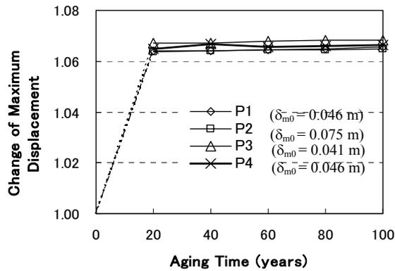
Figure 12: Change of maximum pier displacement
