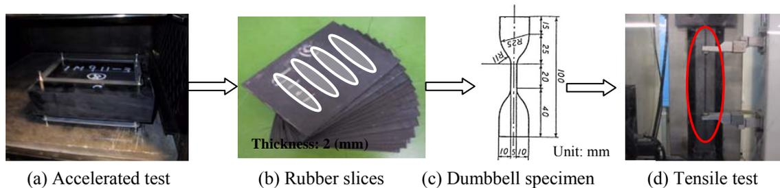
**Figure 1: Accelerated thermal oxidation test flow**
