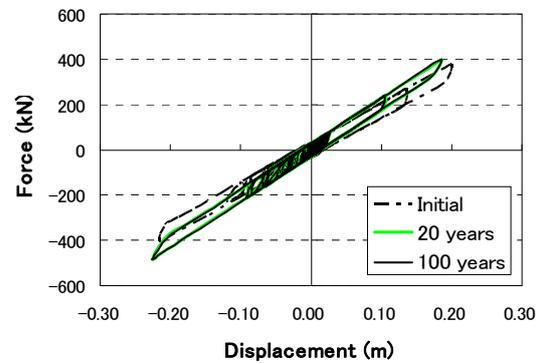
**Figure 11: Hysteretic curve of bearing on Pier 2**
