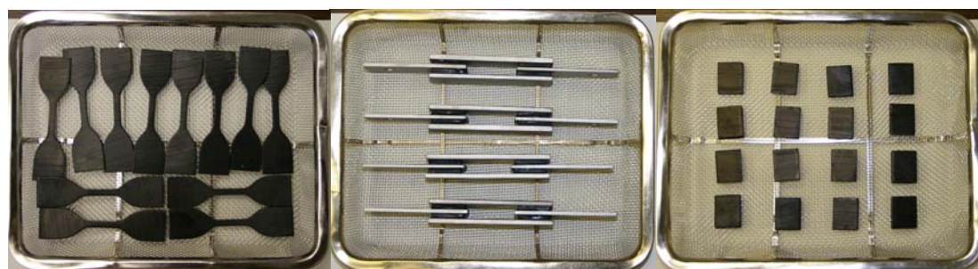
(a) No.3 Dumbbell Specimens (b) Lap-Shear Specimens (c) Lap-Shear Specimens without Metal Plates
