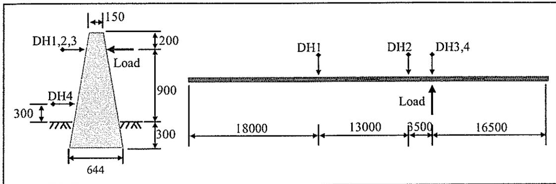
Fig. 2. On-site Full-scale Statistic Loading Tests (unit: mm)
