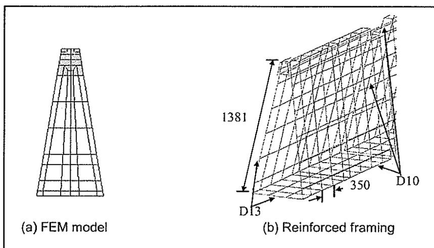
Fig. 8. FEM Models of a Single-slope Concrete Guard Fence
