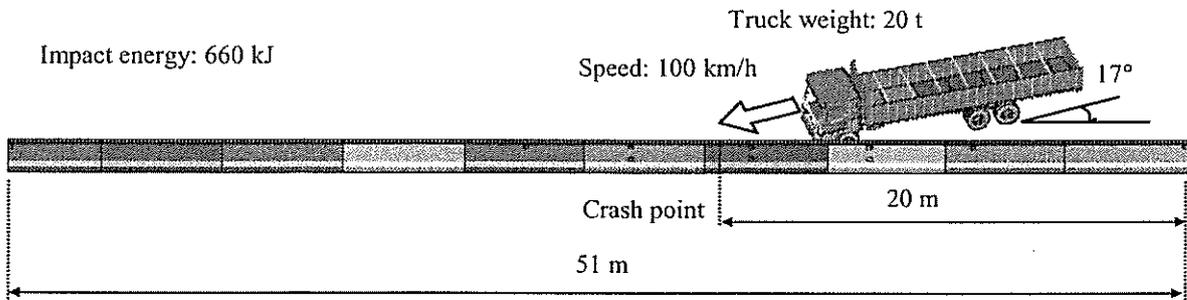
Fig. 6. On-site Full-scale Crash Tests
