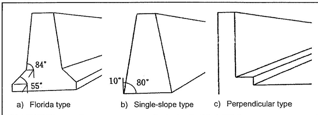
Fig. 1. Typical Concrete Guard Fences
