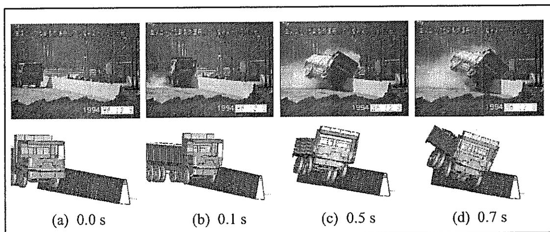
Fig. 9. Impact Performance of a Truck with a Single-slope Concrete Guard Fence
