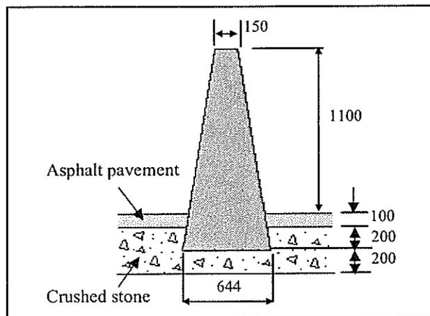
Fig. 3. Cross Section of a Single-slope Concrete Guard Fence
