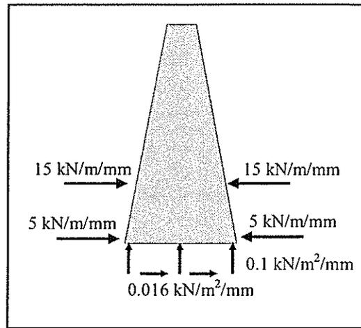
Fig. 4. Spring Models of the Subgrade of a Single-slope Concrete Guard Fence
