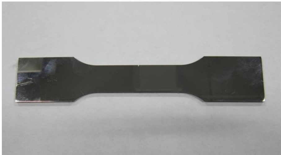
Fig. 2-4 The mirror-surface of a specimen after mechanical polishing.
