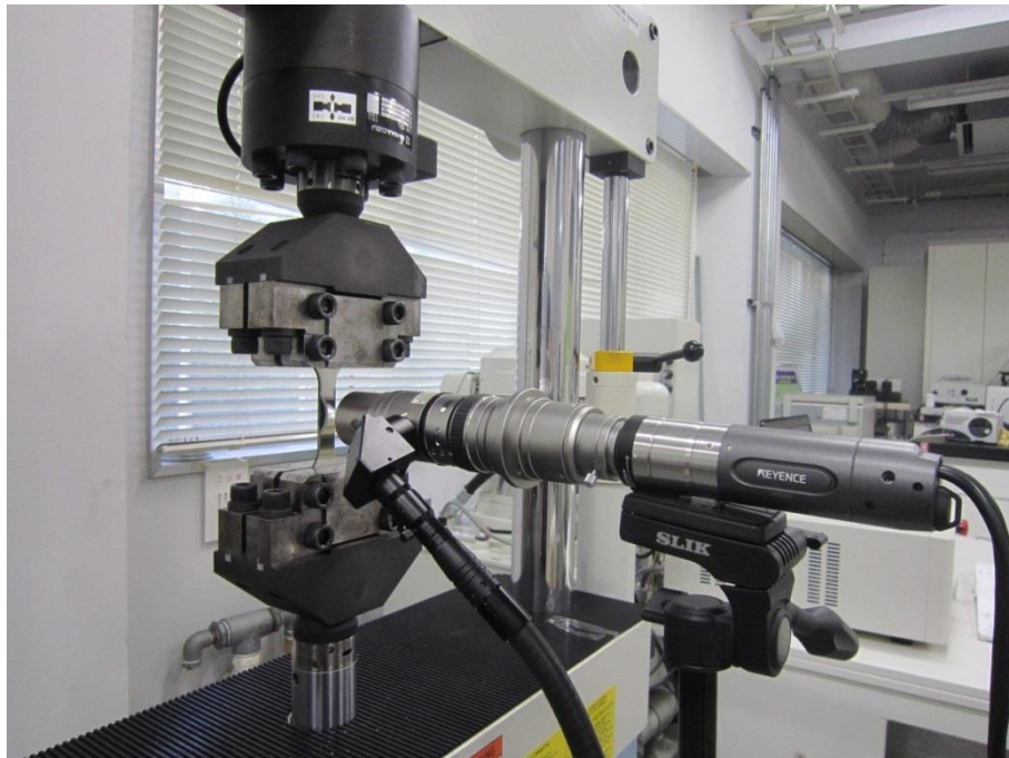
Fig. 2-6 The hydraulic-driven testing machine.
