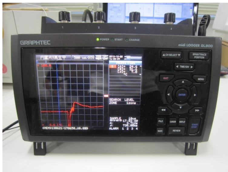
Fig. 2-17 The equipment of temperature measurement (LOGGER GL900).
