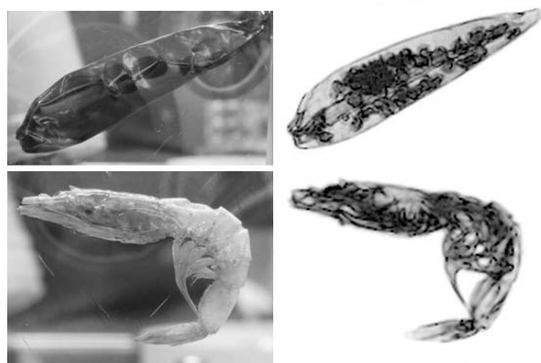
Fig. 1 Spectroscopic THz imaging of dried red pepper and dried shrimp
