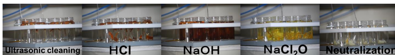
Figure 5-17: Flow chart of chemical cleanings.
