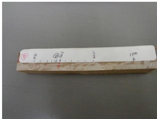
Figure 8-3: Picture of the Hinoki cypress sample. The age determination of this sample was done by T. Mitsutani using the dendro chronology.
