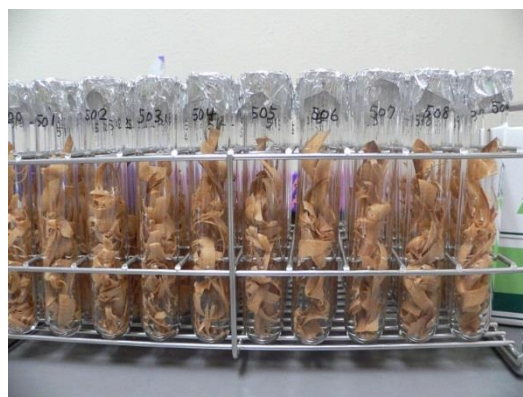
Figure 5-16: Separated wood samples. Each samples in test tubes are annual ring sample.
