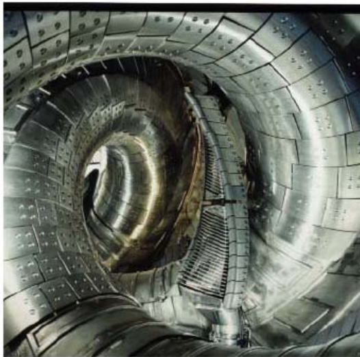
Fig.1 The ICRF antenna used in the experiment. The antenna is located in the toroidal section where the cross section is vertically elongated
