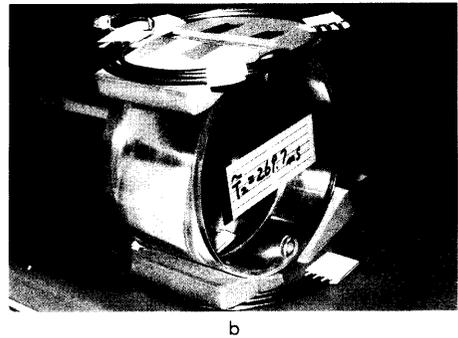
a Fig.1. Diagram of wireless axial pair resonator (WAPR).
