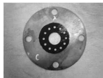
Fig.3 Flange with orifice
