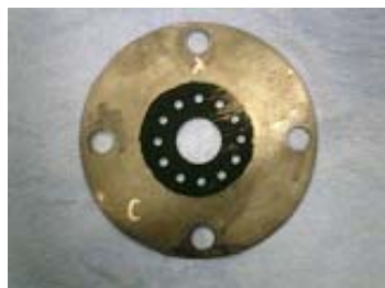
Fig.3 Flange with orifice
