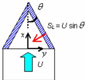
(c) 2D flame on a slot burner
