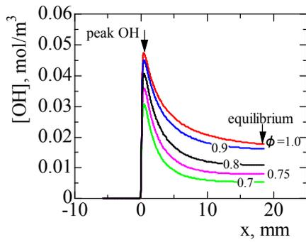
Figure 5 OH profiles of 1D flame in uniform flow at the equivalence ratio of 0.7, 0.75, 0.8, 0.9 and 1.0. There is a peak OH concentration of super-equilibrium value in flame region. At downstream, its concentration becomes equilibrium value.
