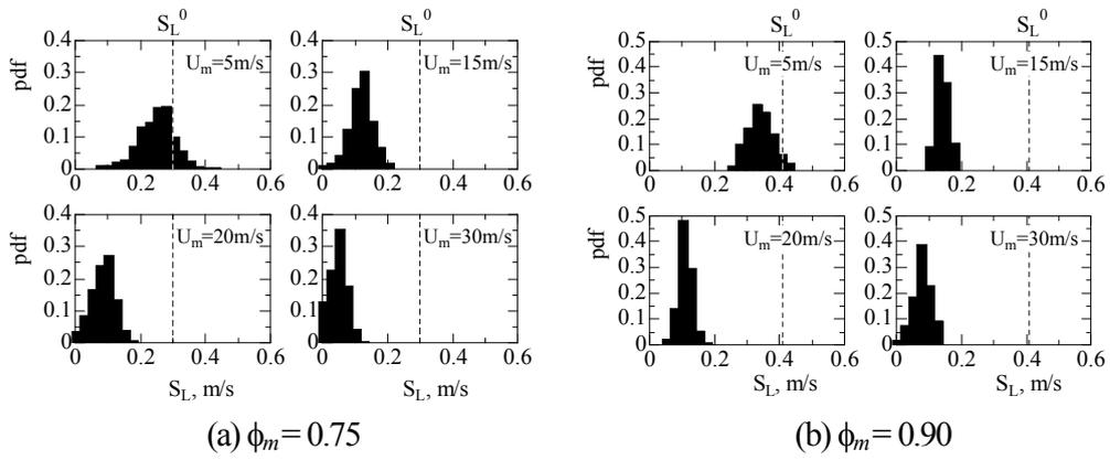
Figure 11 PDF of local burning velocity for (a)  $\phi_m = 0.75$  and (b)  $\phi_m = 0.90$ . For comparison, the laminar burning velocity,  $S_L^0$ , is shown by dotted line.
