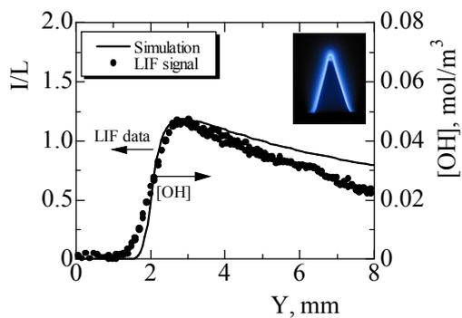
Figure 9 Profiles of LIF signals and simulated OH concentration of flame on a slot burner;  $Z = 10$  mm,  $\phi = 0.9$ .
