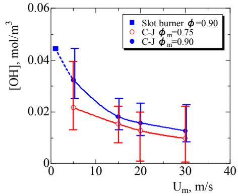
Figure 10 Variations of peak OH concentration with exit velocity. Measured maximum and minimum are shown by error bar.
