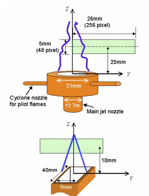
Figure 2 Cyclone-jet combustor (upper) and slot burner (lower).
