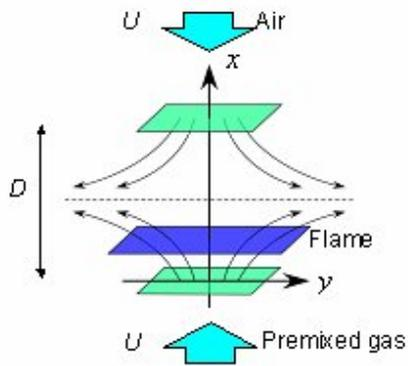
(b) Counter-flow flame in opposed jets of premixed gas and air
