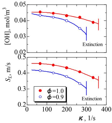
Figure 6 Peak OH concentration and burning velocity of counter-flow flames for  $\phi=0.9$  and 1.0.
