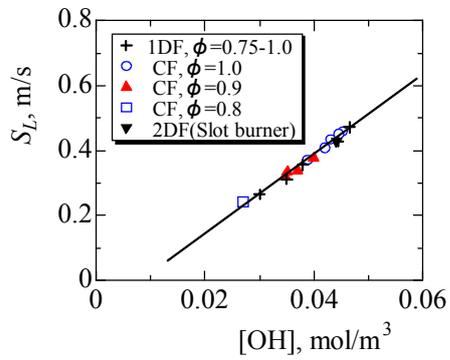
Figure 7 Relationship between peak OH concentration and burning velocity in counter-flow premixed flame for propane/air mixtures. All the computed data of 1D flame in uniform flow and laminar flame on a slot burner are plotted.
