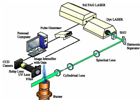
Figure 3 Experimental setup for OH-PLIF system.
