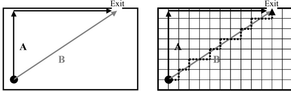
Fig. 2 Example for evacuation toward the exit, with two paths of A and B. Left figure is movement in real situation without grid points, and right figure shows one with CA grids.
