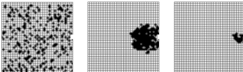
Fig. 6 Evacuation simulation in a large room with one exit. Three typical stages are shown; (a)  $t = 0.5$  s, (b)  $t = 25$  s, and (c)  $t = 52.5$  s.
