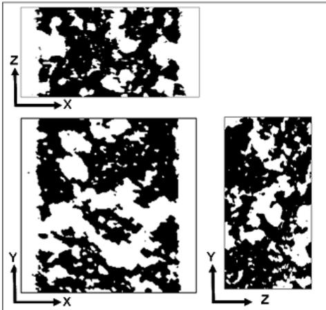
Figure 1 CT images of the filter are shown. The image area is  $400\ \mu\text{m}$  ( $x$ )  $\times$   $400\ \mu\text{m}$  ( $y$ )  $\times$   $200\ \mu\text{m}$  ( $z$ ). Complex porous structure with variety of pore size is well observed.
