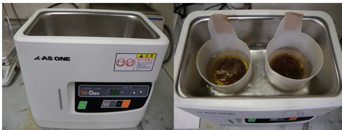
Figure 5.2.12 Ultrasonic bath and lift-off process.
