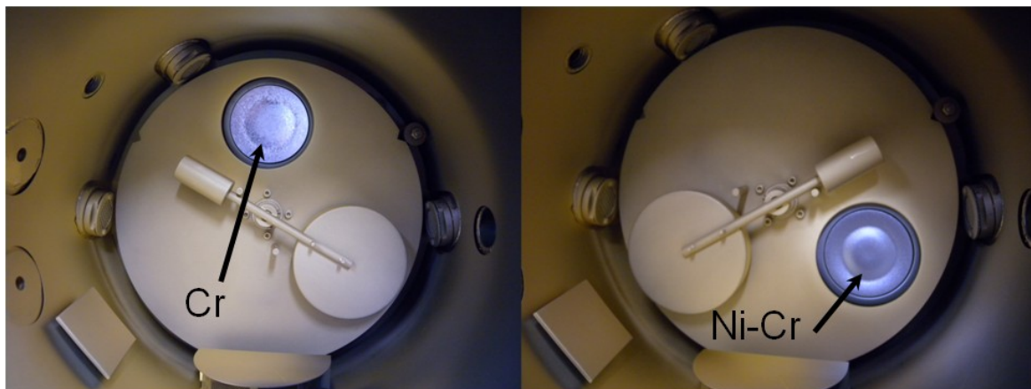
Figure 5.2.10 Cr target and Ni-Cr target inside the sputtering chamber.
