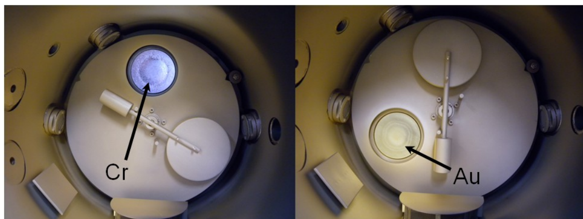
Figure 5.2.16 Cr target and Au target inside the sputtering chamber.
