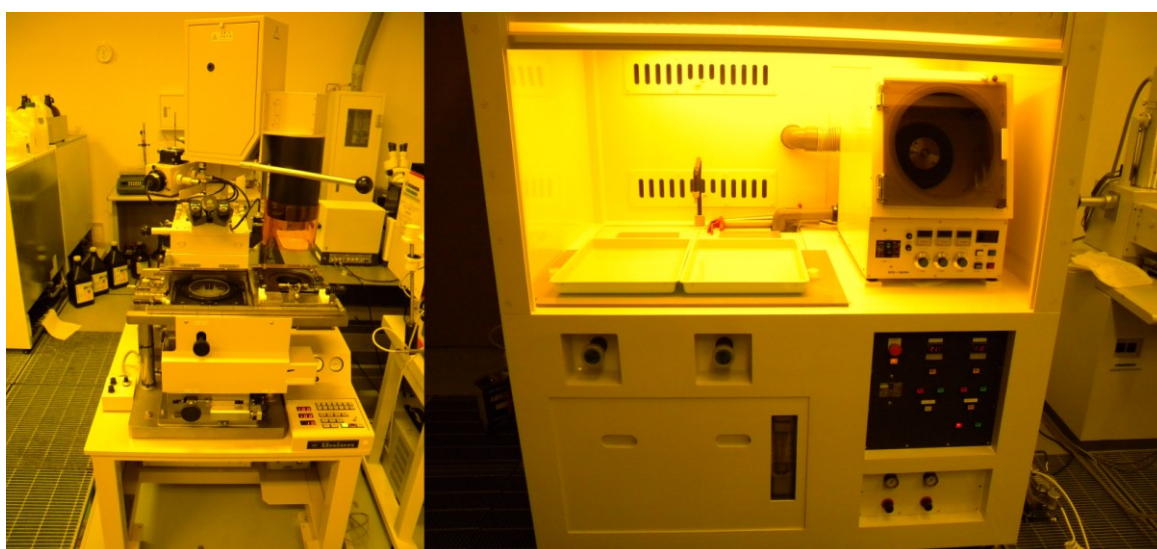
Figure 5.2.5 PEM-800 mask aligner and wet-bath for development.
