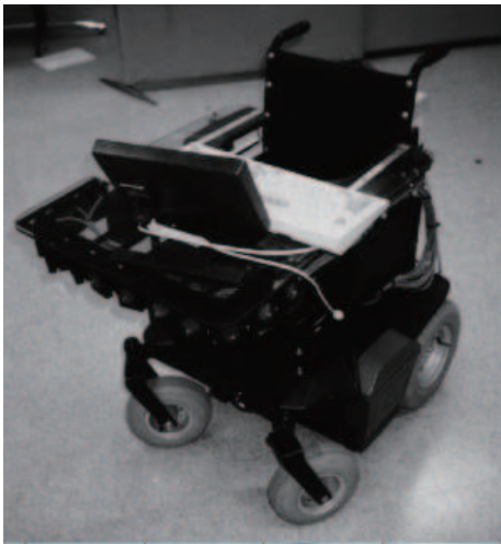
(C) The NavChair Assistive Wheelchair Navigation System
