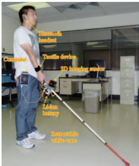
(c) Dr. Cang Ye is working to develop a “smart cane” that will help visually impaired people travel more easily and safely. [41]
