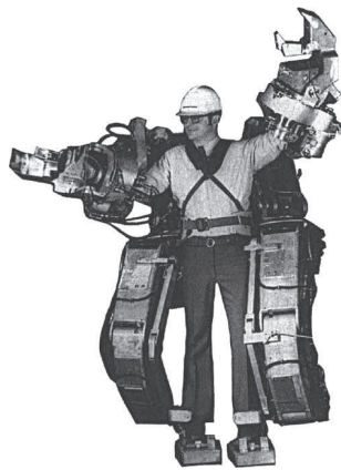
(b) The Hardiman exoskeleton prototype, developed in the 1960s by General Electric.
