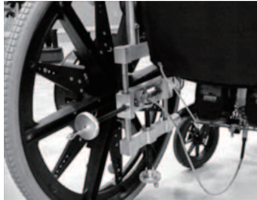
(B) Quick-adjust wheelchair axle. Position of axle changed in vertical and horizontal directions with turn of knob
