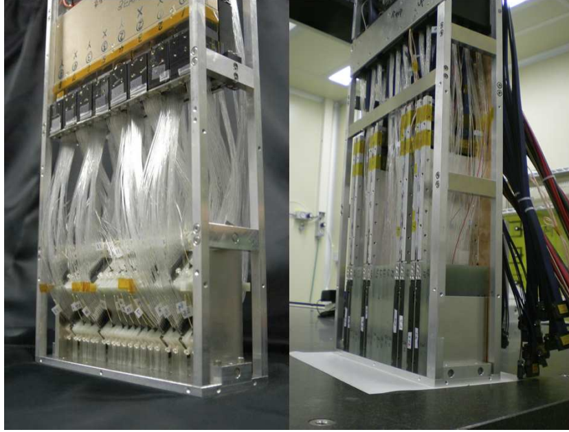
Figure 2.7: Pictures of the LHCf detectors. Left panel shows the Arm1 detector, and right shows the Arm2 detector.
