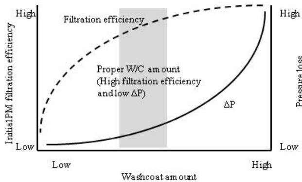
**Figure 17 Diagram of relationship between W/C amount and pressure loss, initial PM filtration efficiency**
