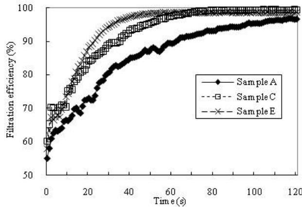
**Figure 7** Number-based filtration efficiency upon initial usage for DPF samples A, C, and E
