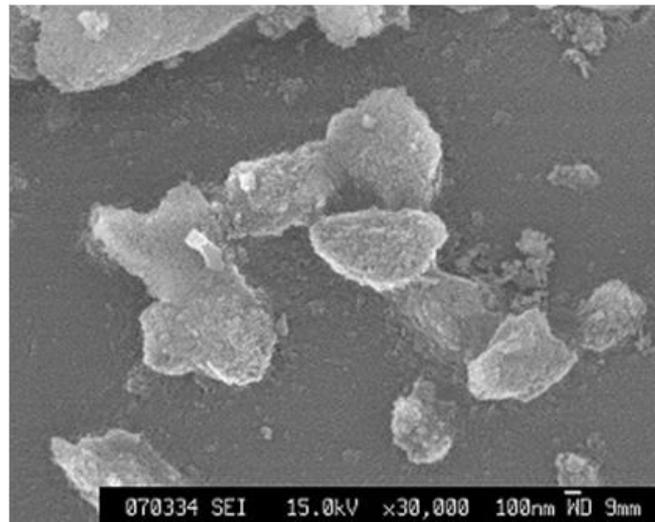
**Figure 6 SEM image of  $\gamma$ -alumina particles**
