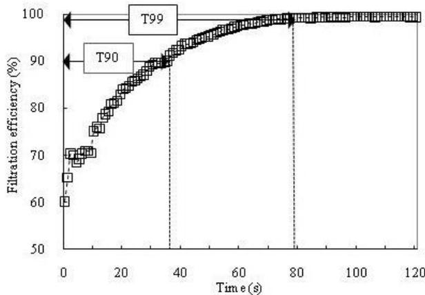
**Figure 8** Time-variation of filtration efficiency with parameters of T90 and T99; T90 is the time to reach more than 90% filtration efficiency, and T99 is the time to reach more than 99% filtration efficiency, from initial filtration usage
