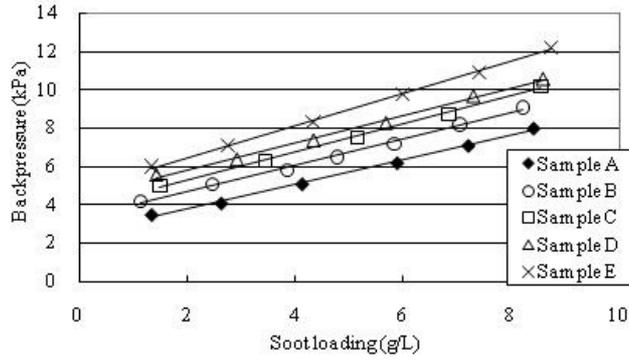
Figure 13 Backpressure during soot loading for all samples
