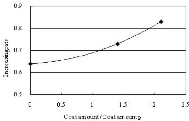
Figure 14 Increasing rate, which is the slope of the backpressure in Fig. 13, during soot loading for samples A, C, and E
