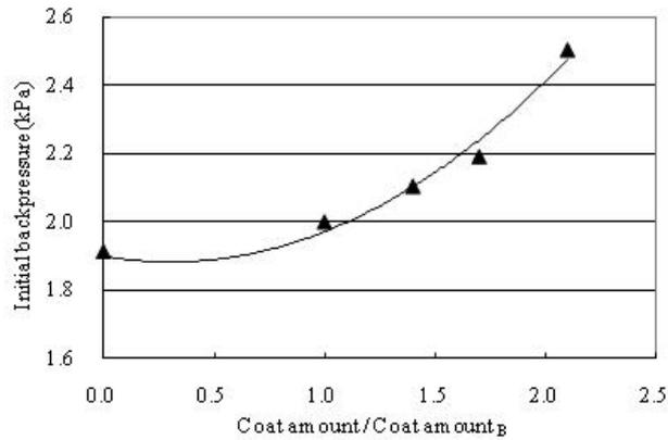
**Figure 12 Relationship between W/C amount and initial backpressure (no PM loading)**
