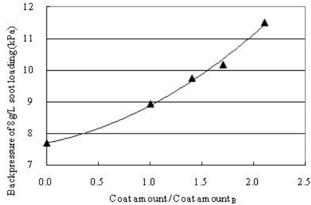
**Figure 16 Relationship between backpressure of 8g/L soot loading and W/C amount**
