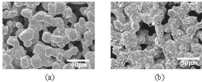
*Figure 1 SEM image of (a) wall surface of uncoated DPF, (b) wall surface of W/C DPF*
