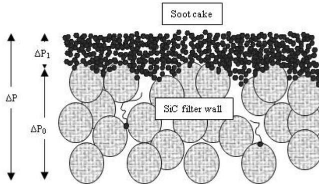
Figure 15 Image of total pressure loss during soot loading;  $\Delta P$  is total pressure loss,  $\Delta P_0$  is initial pressure loss across filter wall, and  $\Delta P_1$  is pressure loss caused by soot cake
