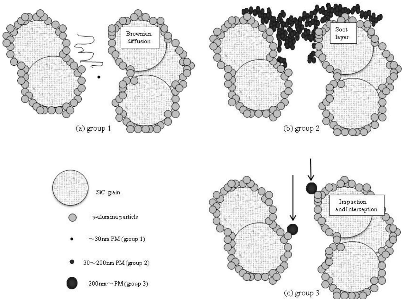
**Figure 11 Particle trap mechanism classified according to PM size**
