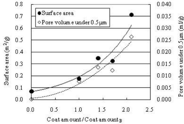
**Figure 5 Relationship between W/C amount and surface area per unit mass of the filter wall, pore volume under 0.5 μm**
