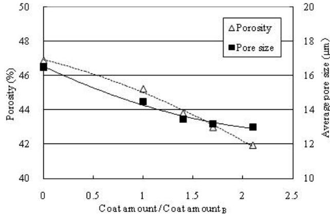
**Figure 3** Variations of porosity and average pore size with W/C amount
