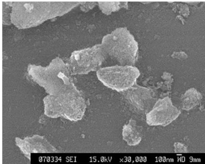
**Figure 6 SEM image of  $\gamma$ -alumina particles**
