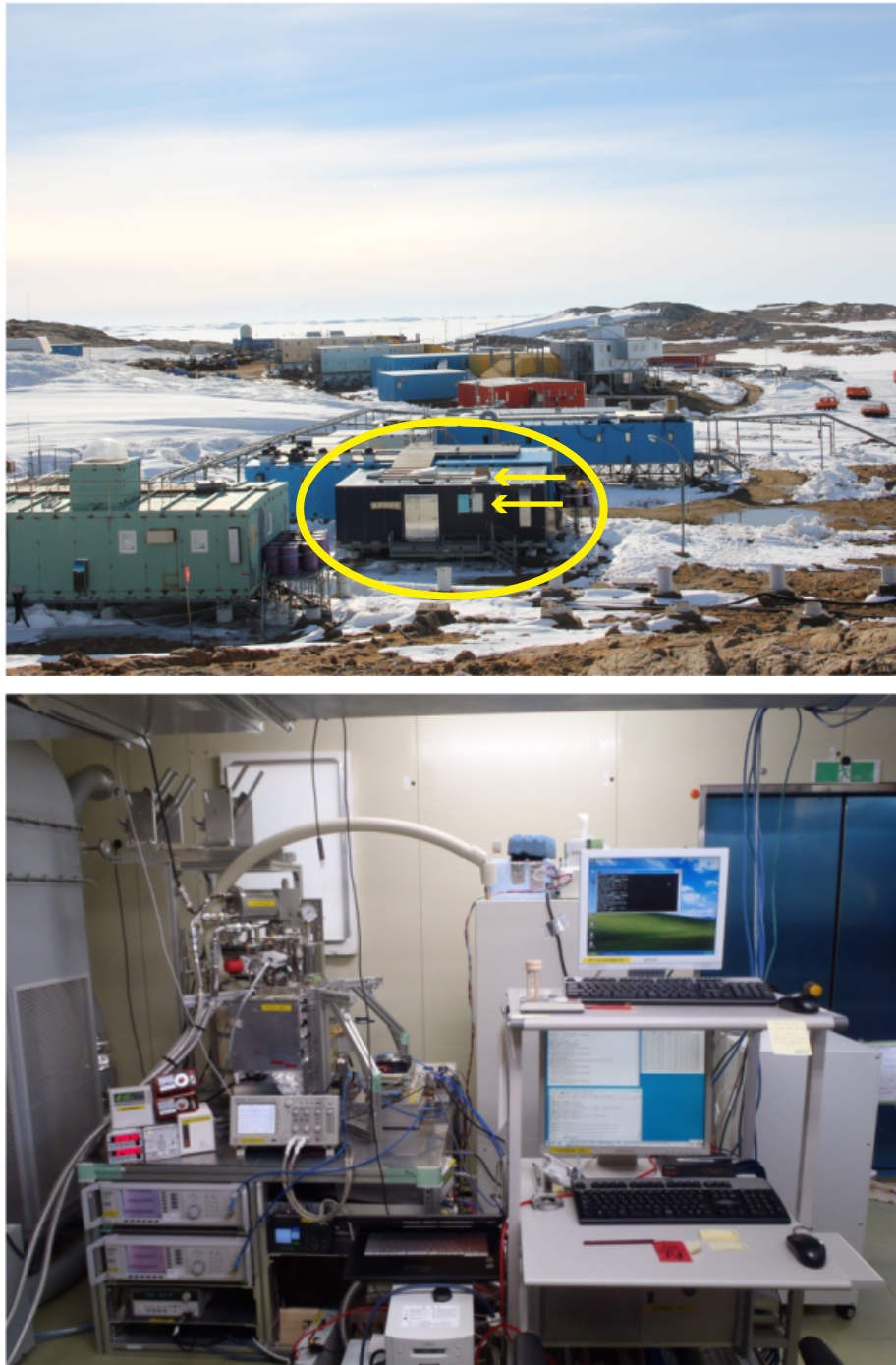
Figure 2.3 (top) The main area of the Syowa station. A yellow circle indicates the optical observation building and yellow narrows indicate the observation windows which are facing south and the zenith are made of polystyrene. (bottom) The millimeter-wave spectroscopic radiometer in the optical observation building.
