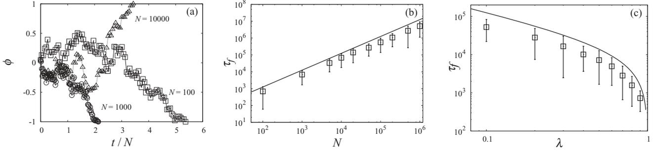
FIG. 6. (a) Time evolution of  $\phi$  in the Monte Carlo simulation. (b) The conversion time for various system size  $N$ . (c) The conversion time for various decay rate  $\lambda$ . The solid lines represent the estimated conversion time using the simplified model Eq. (20).
