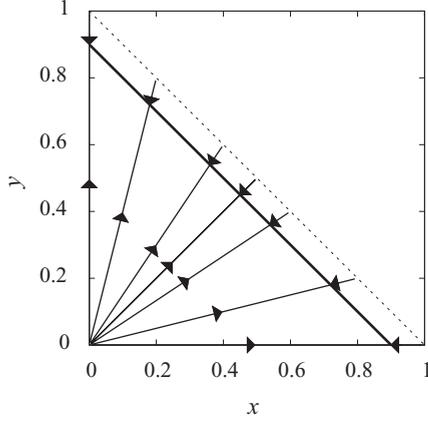
FIG. 1. Flow diagram of Eqs. (2) and (3). The thick solid line,  $x + y = 0.9$ , represents the fixed line.
