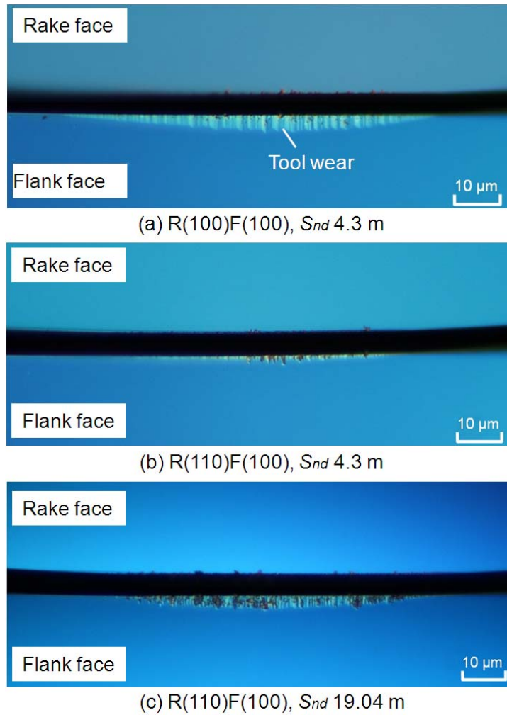
Fig. 3.17 Microphotographs of cutting edges with different crystal orientations (R: rake face, F: flank face, S_{nd} : nominal cutting distance)
