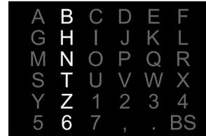
Fig. 1. User-interface while the second column is intensified.
