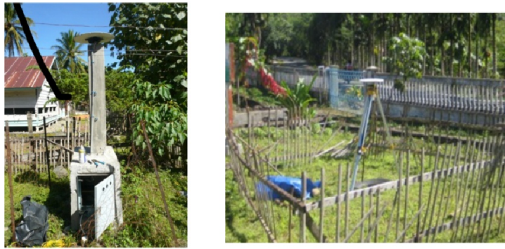
Figure 3.6. Typical GPS measurements in northern Sumatra. (Left-hand side picture) A concrete pillar type for continuous GPS sites. (Right-hand side picture) Campaign GPS measurements using tripod.
