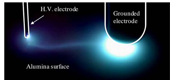
Figure 4. Still image of surface flashover. ( $-28$  kV impulse)
