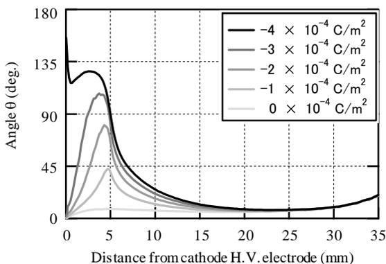
**Figure 9.** Incident angle of lines of electric force to alumina surface (applied voltage: -28 kV, area A:  $0 \text{ C/m}^2$  to  $-4 \times 10^{-4} \text{ C/m}^2$ ).
