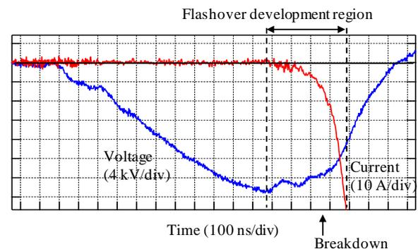
Figure 5. Surface flashover waveforms.
