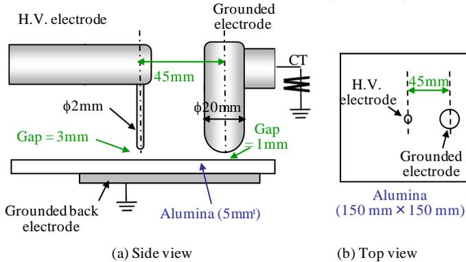
Figure 2. Electrode configuration.
