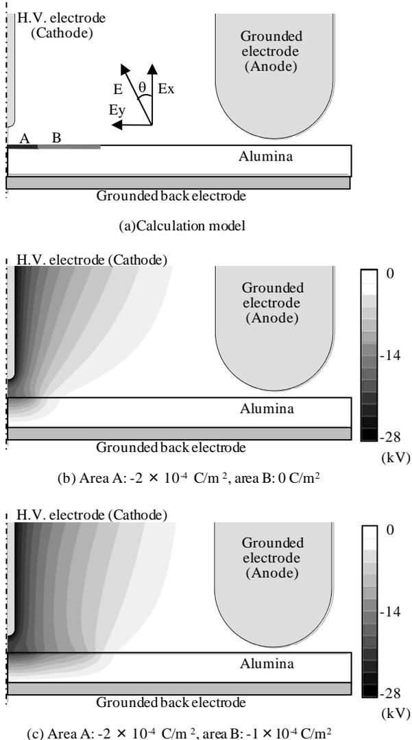
**Figure 8.** Calculation result of equi-potential distribution when negative charging exists (applied voltage: -28kV).
