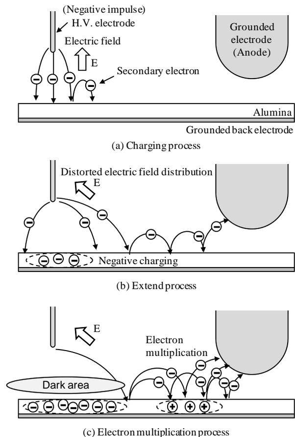
**Figure 7.** Estimation of surface flashover initiation and forming dark area mechanism.
