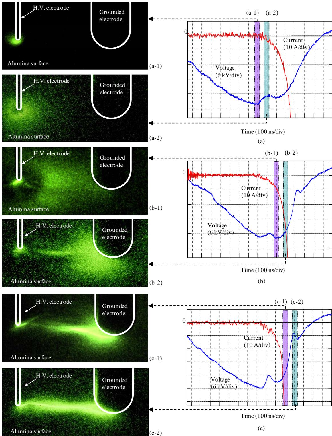
**Figure 6.** Fast-framing image and surface flashover waveforms
