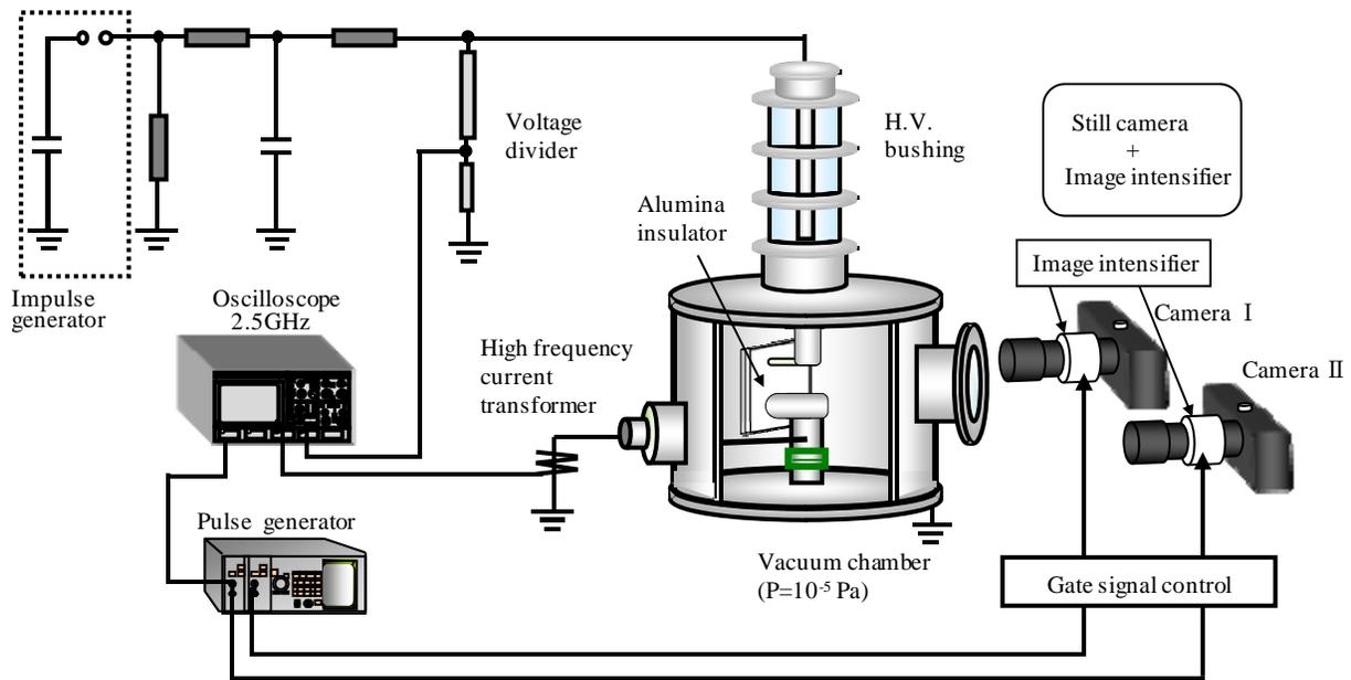
Figure 1. Experimental setup and measuring systems.
