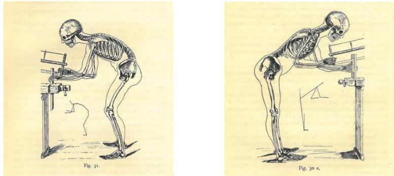
*Figure 2* The images show the correct and incorrect working positions for sawing.
