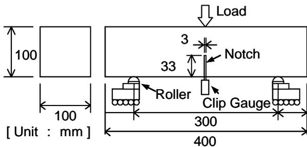
Fig.1 Shape of Specimen (Series 1)
