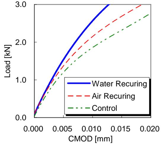
(a) Difference of the initial stiffness at the second loading depending on recuring condition
