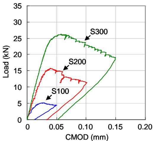
Fig.10 Load-CMOD Curve of S100, S200 and S300
