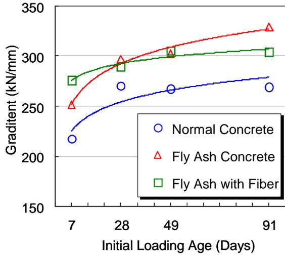
Fig.4 The Initial Stiffness at each Loading Age
