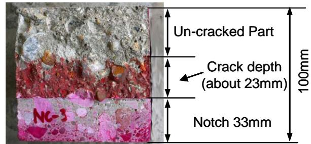
Fig.3 Crack Depth of CMOD 0.05mm
