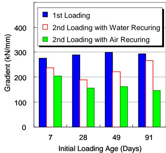
Fig.8 Difference of Gradient by Loading Process (Fly Ash Concrete)
