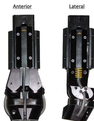
Figure 3.1 Anterior and lateral view of POLAR II original knee joint (left knee)
