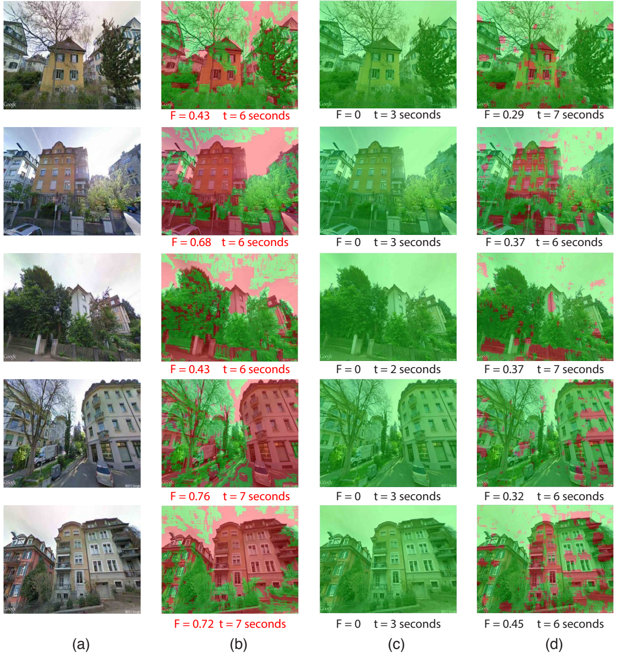
Figure 4.7: Segmentation of natural and man-made structures for samples of the Google Street View image dataset. (a) Original images. These images exhibit “blocking” artifacts. (b) Proposed method. (c) Conditional random field approach [83]. (d) Mean squared error approach [84]. Image regions highlighted with the color green indicate nature-made structures. Image regions highlighted with the color red indicate man-made structures.
