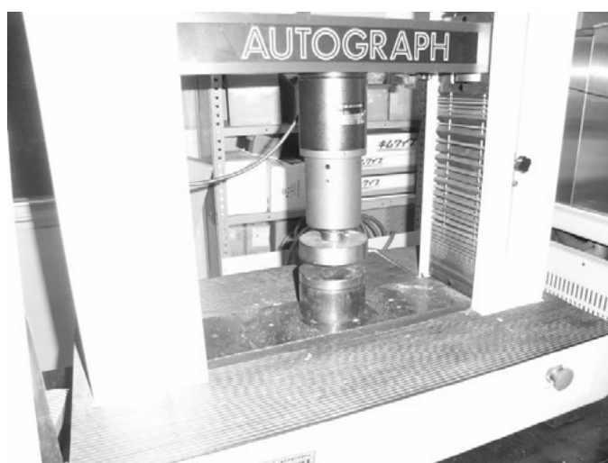
Fig. 4-3 Mechanical testing machine and compression test equipment.
