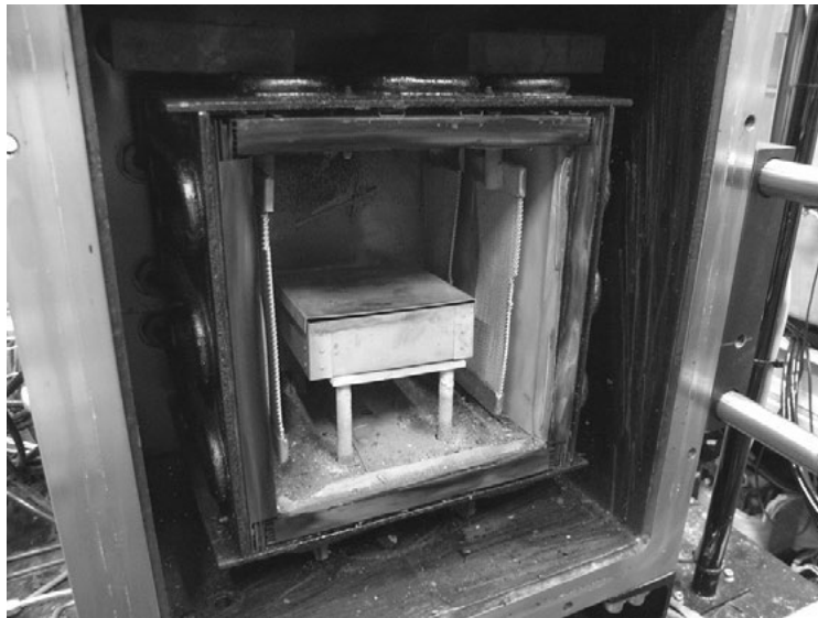
Fig. 2-5 Vacuum furnace used to sintering porous titanium.
