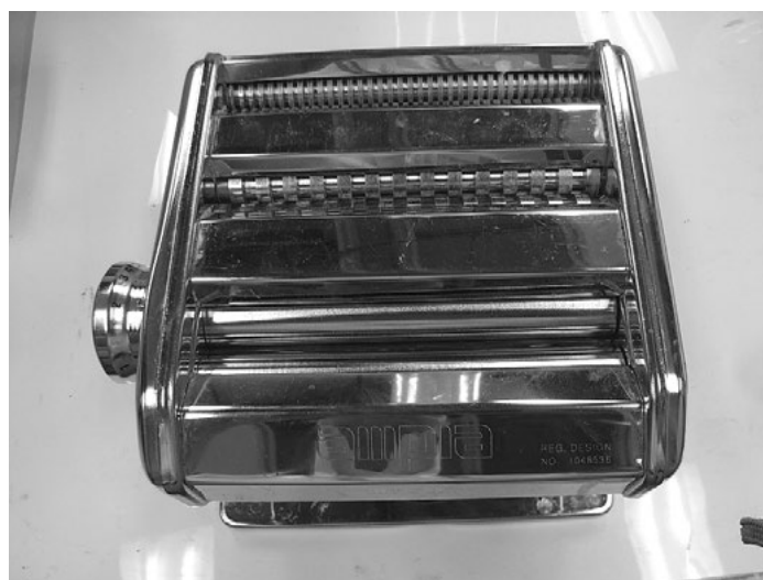
Fig. 2-3 Pasta machine used to roll the compound.
