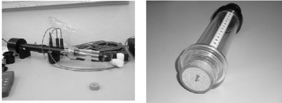
Fig. 6-6 Sound absorption measurement equipment for impedance tube method.
