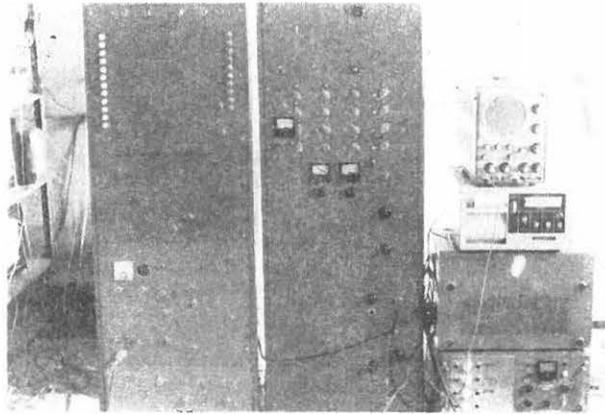
Photo. 2a Time signal generator and waveform recorder for ELF
