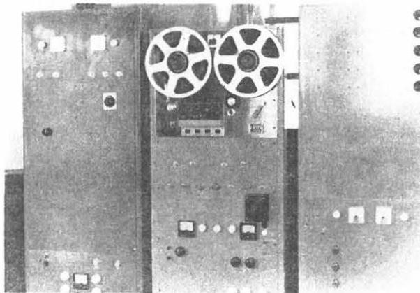
Photo. 2b Receivers for the measurement of integrated field intensity of atmospherics and waveform recorder for Schumann resonance
