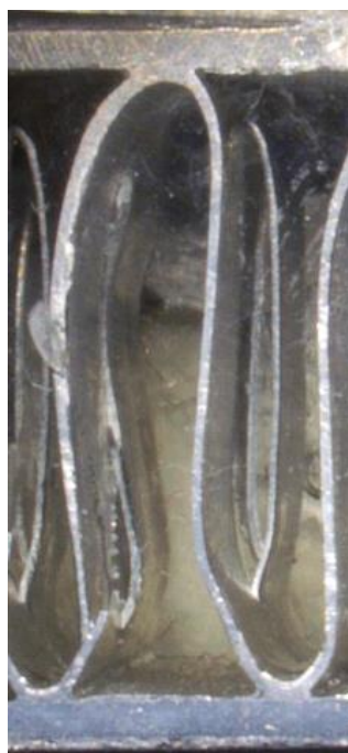
Fig. 2. 4 Cross section of inner fin of intercooler.
