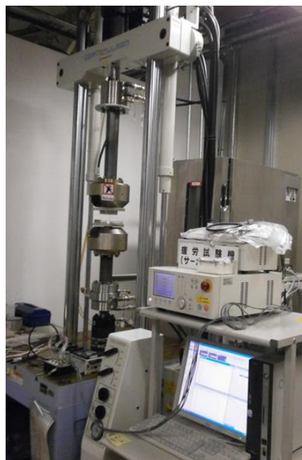
Fig. 3. 7 Testing machine used for compression test; EHF-50kN.
