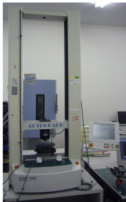
Fig. 4. 9 Testing machine for four-point bending test; AG-IS10kN.
