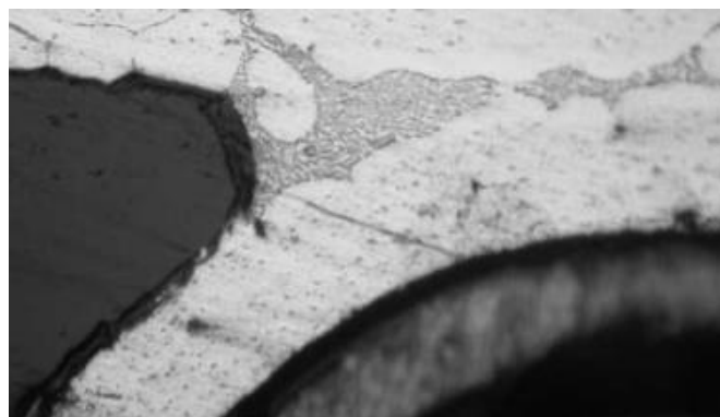
Fig. 2. 5 Enlarged view of brazing fillet.
