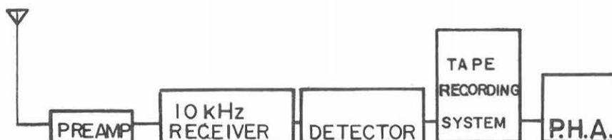
Fig. 1 Block Diagram of The Instrument
