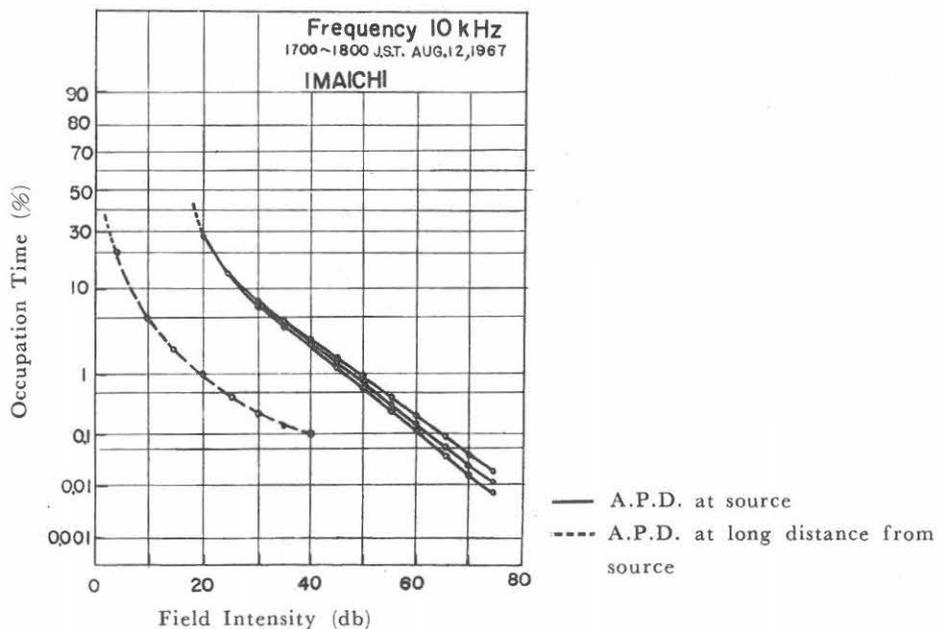
Fig. 2 Amplitude Probability Distribution of Atmospheric Radio Noise at Source.
