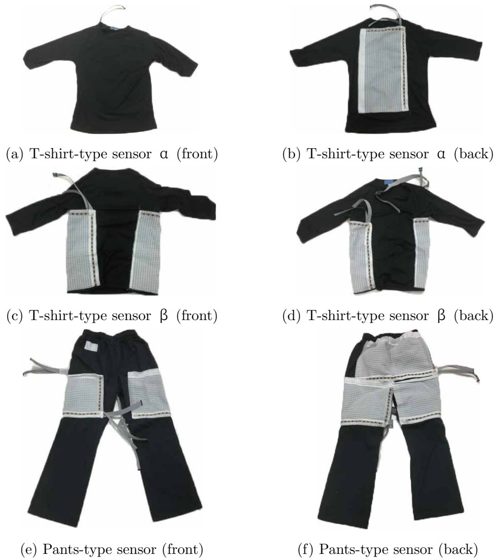
Figure 3.6.1: Prototype I: a prototype for body surface contact pressure measurement using commercial garment
