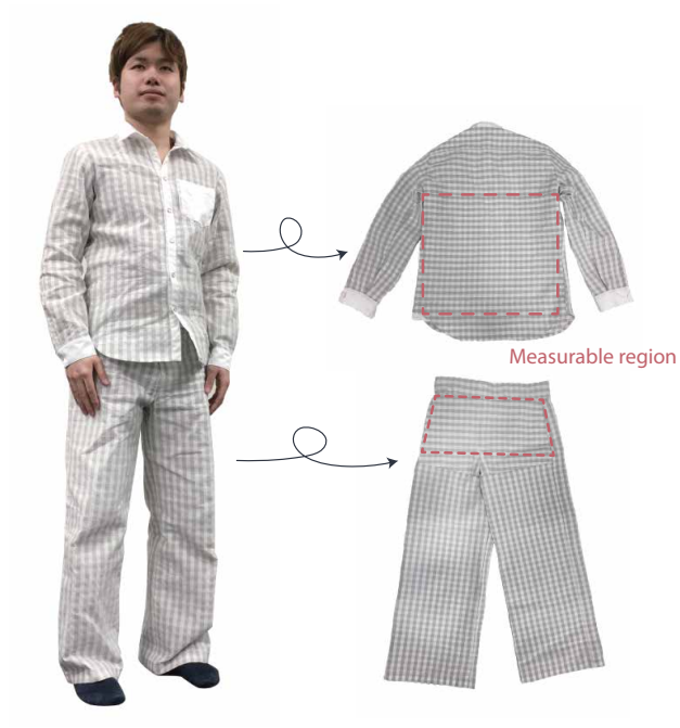
Figure 1.2.1: Garment-type pressure sensor using the textile pressure sensor
