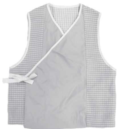
(a) Jinbei-type sensor (jacket, front)
