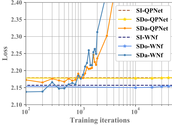
Figure 5.14: Validation losses of different vocoders ( SI : speaker-independent; SD : speaker-dependent; o : only update output layers; a : update whole network).
