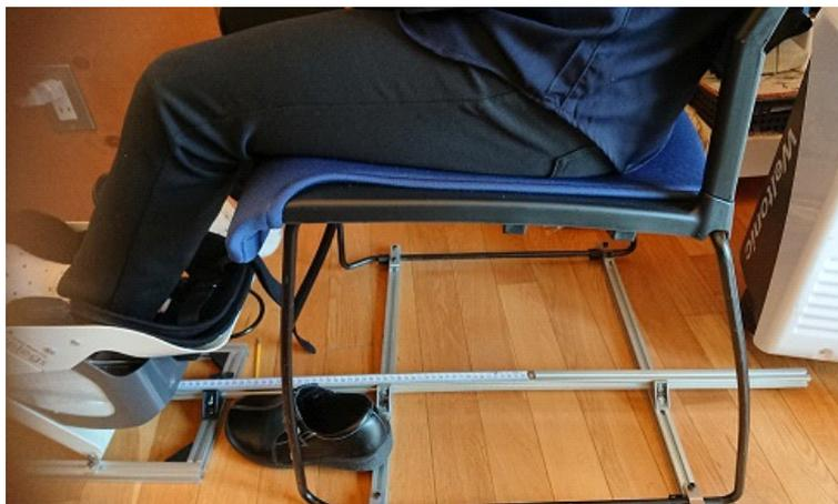
Fig. 3.17: Stretching machine connected chair using metal frame
