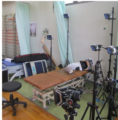
Fig. 2.8: Experimental apparatus of three-dimensional motion analysis
