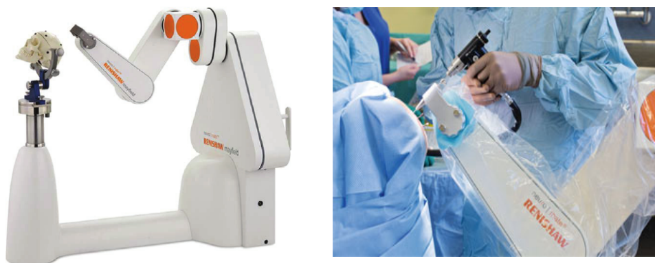
Figure 1.14: Current version of Neuromate robotic system used for stereotactic surgery. (Reprinted with permission from Zanotto et al. [65])
