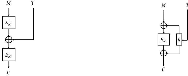
Figure 5.1: The LRW constructions. LRW1 is depicted on the left, and LRW2 is depicted on the right.
