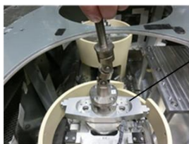
FIG. 2.3 Excitation system including the force measurement system, with eccentric circulate motion motors, load cells, excitation bases, and support springs.
