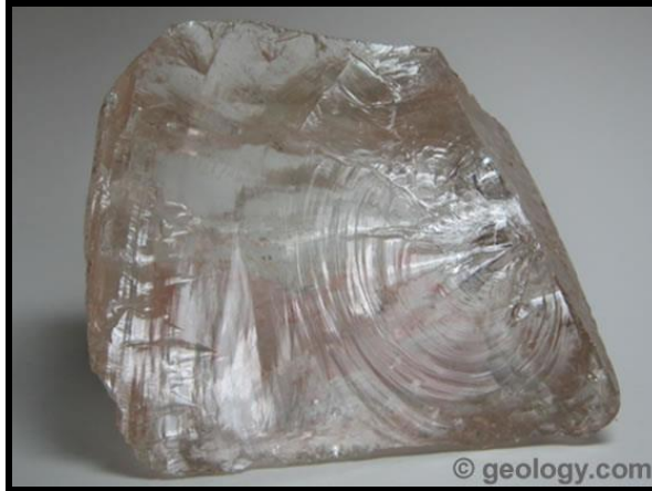
Conchoidal fracture (quartz)
