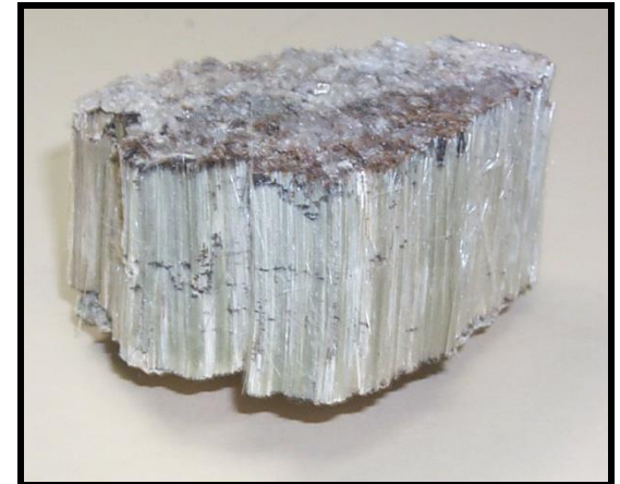
Splintery fracture (Asbestos = fibrous silicates minerals)
