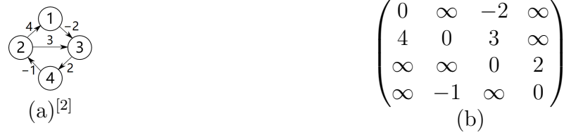
Fig. 4.27. (a) an oriented graph with negative edges; (b) the matrix M^0 listing the weight of its all edges.
